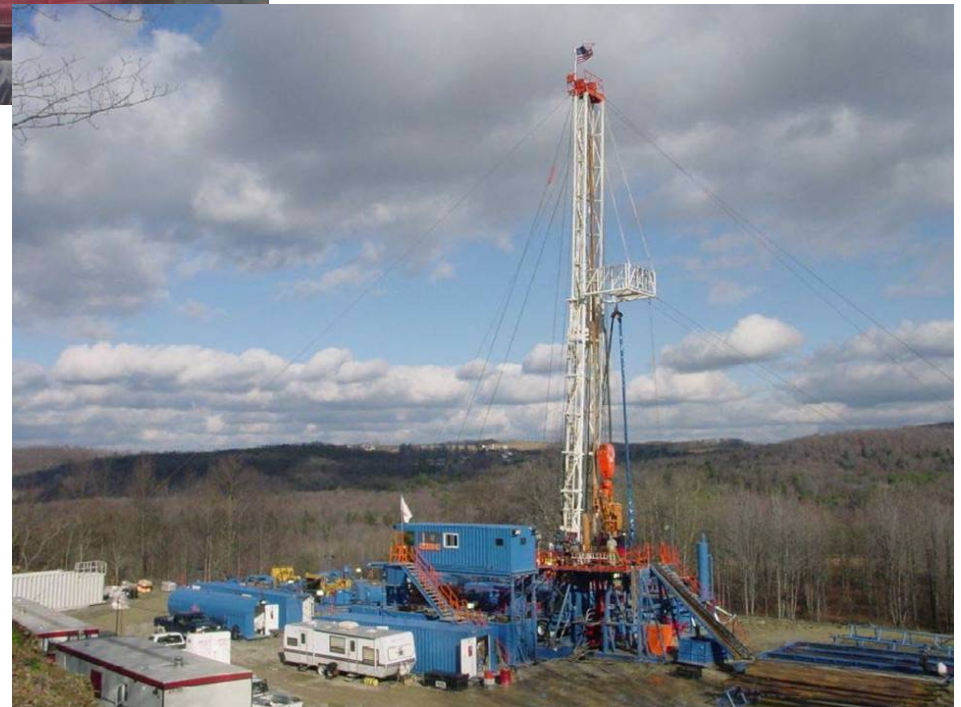
Directional rig for drilling horizontal leg
